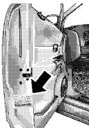
This label contains the month and year of manufacture, Gross Vehicle Weight Rating (GVWR), Gross Axle Weight Rating (GAWR) front and rear, and Vehicle Identification Number (VIN). A Month-Day-Hour (MDH) number is included on this label and shows the Month, Day, and Hour of manufacture. The bar code that appears on the bottom of the label is your Vehicle Identification Number (VIN).
